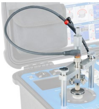
◀ CV-10 with adapter for proximity probes
