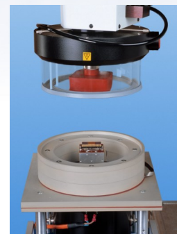
Vibration testing of small modules under Thermostream®
