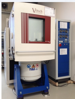
Vibration testing system with climate chamber
