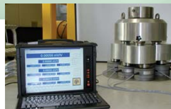
Modern force multiplication: Build-up 9 \cdot 600 \text{ kN} = 5.400 \text{ kN}
