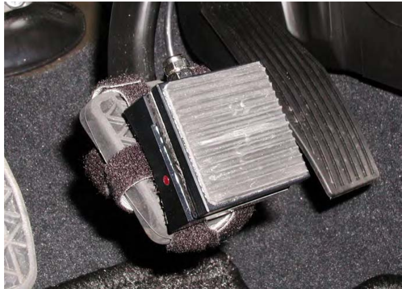
PFS fitted to Brake Pedal
