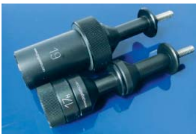
Clamp and Magnetic Holder lengthened by 45mm
